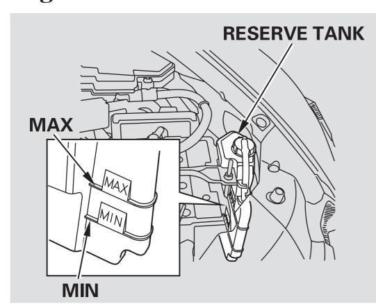
Look at the coolant level in the radiator reserve tank. Make sure it is between the MAX and MIN lines. If it is below the MIN line, see **Adding Engine Coolant** on page 192 for information on adding the proper coolant.
