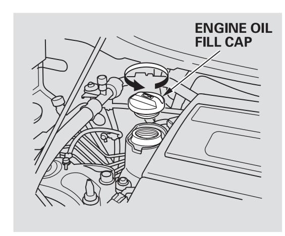
Unscrew and remove the engine oil fill cap on the valve cover. Pour in the oil slowly and carefully so you do not spill any. Clean up any spills immediately. Spilled oil could damage components in the engine compartment. Reinstall the engine oil fill cap, and tighten it securely. Wait a few minutes, and recheck the oil level on the engine oil dipstick. Do not fill above the upper mark; you could damage the engine.
