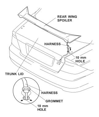
8. Position the trunk spoiler onto the trunk lid, and install the four cap nuts. Torque the cap nuts to 7 to 10 N•m (5 to 7 ft-lb).
