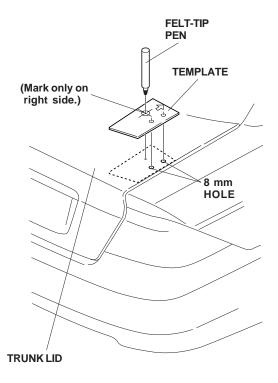
Remove the template, and lightly center-punch the mark.
