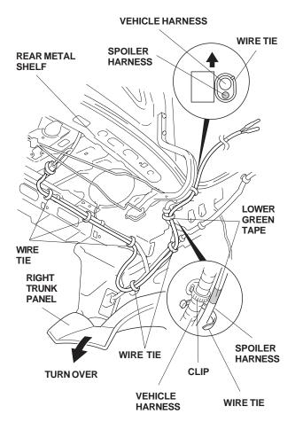
19. Route the spoiler harness alongside the vehicle harness, and secure it with six wire ties in the areas shown.
