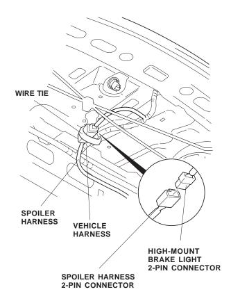
17. Secure the 2-pin connector to the vehicle harness with one wire tie in the area shown.
