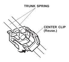
11. With an assistant holding the trunk lid open, remove the old trunk springs from the trunk lid hinge using the special tool. Wear heavy gloves to protect your hands, and pull the special tool slowly and carefully toward you.
