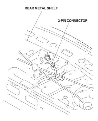
15. Route the 2-pin connector from the high-mount brake light above the trunk springs, and plug it into the 2-pin connector of the spoiler harness.
